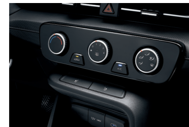
Manual air conditioning system
