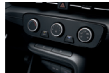
Manual air conditioning system
